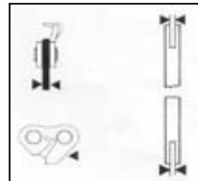
**LINK COUNT:** This enables us to send you the proper length of chain. Mark one drive link, then count drive links around the loop until you return to first link. Your total is the link count.
